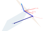
Fig. 2: An example of the torsion calculation for the backbone curve. The cross products in red give two planes. The torsion is then the cosine of the angle between these two planes.
